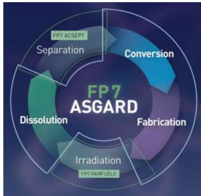
**Figure 1** The ASGARD project in relation to the steps in a circular nuclear fuel cycle and in relation to other important projects in the domain.
